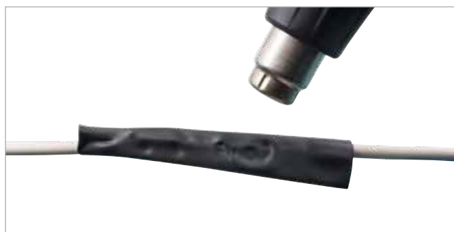
4- Chauffez la gaine thermorétractable
